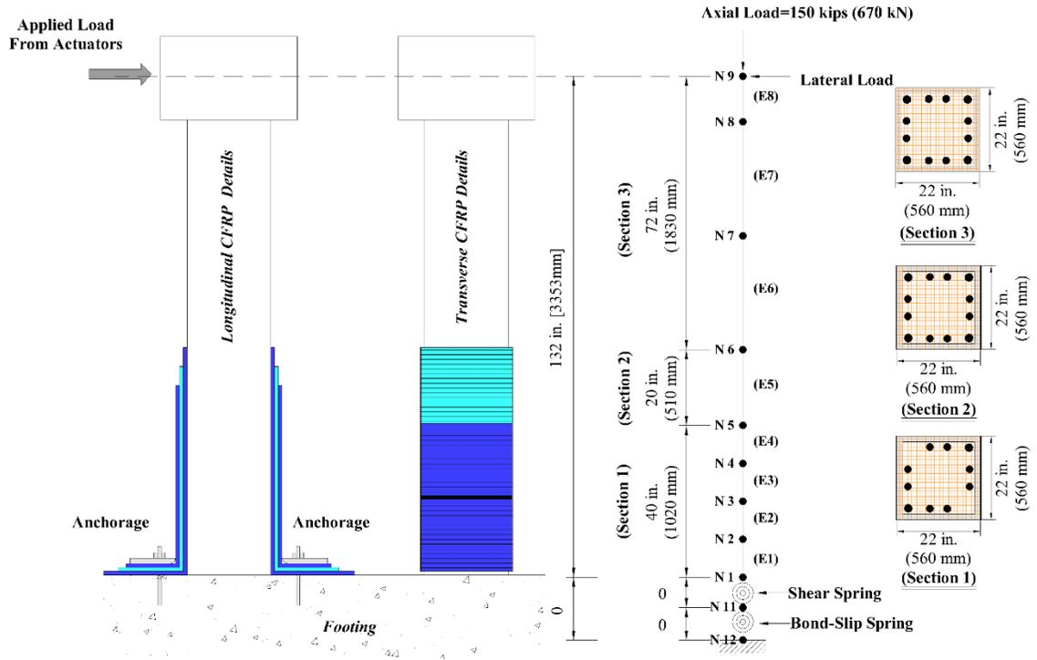
Figure 7 Numerical model for repaired column
