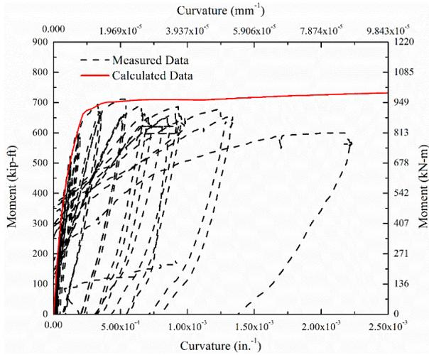
Figure 3 Comparison of measured and calculated moment-curvature relationships for original column
