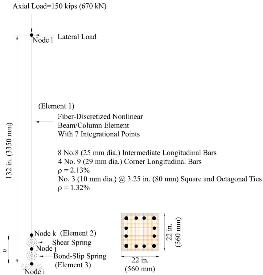
Figure 4 Numerical model for original column
