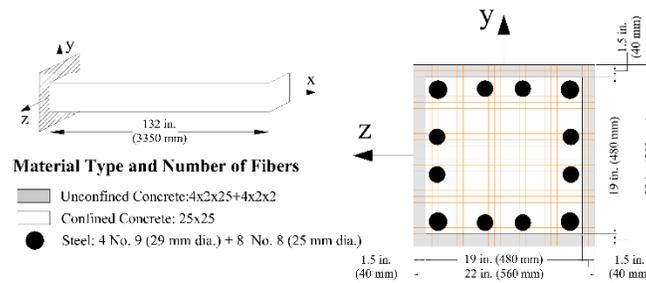
Figure 2 Fiber discretization of the cross-section
