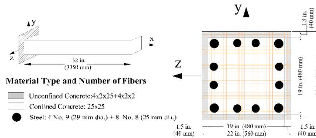
Figure 2 Fiber discretization of the cross-section
