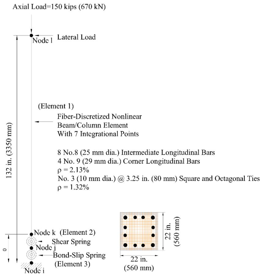
Figure 4 Numerical model for original column
