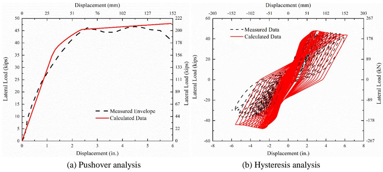
Figure 8 Comparison of the measured and calculated response for repaired column
